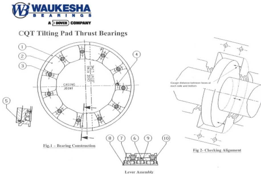
The CQ tilting pad thrust bearing consists of a number of thrust pads (item 2) supported in a cage ring (item 1). Each pad is loosely retained by pad stops (item 3) so that each pad is free to tilt and it is supported on a system of levers (item 7) to equalise load sharing between the pads. A screw held spacer plate (item 8) is fixed to the back face of the cage ring, securing the levers within the cage ring.
