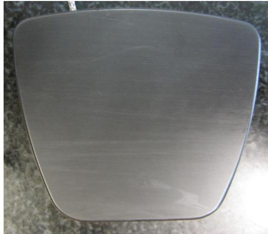
**Figure 5.** PEEK lined pad after test, 11,000 rpm.
