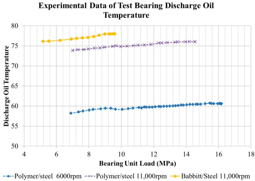
Figure 9. Oil discharge temperature at different speeds.
