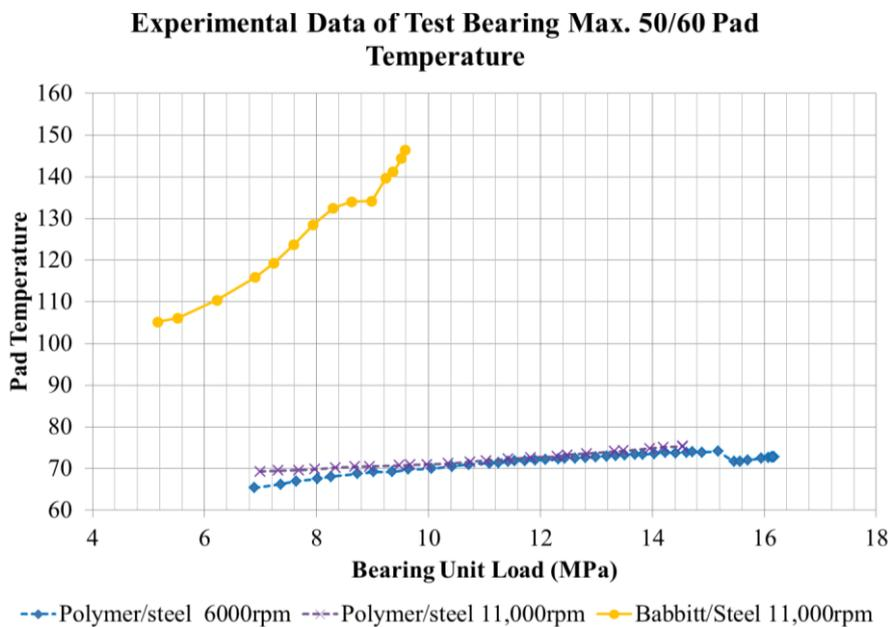
Figure 10. Pad temperature versus load.
