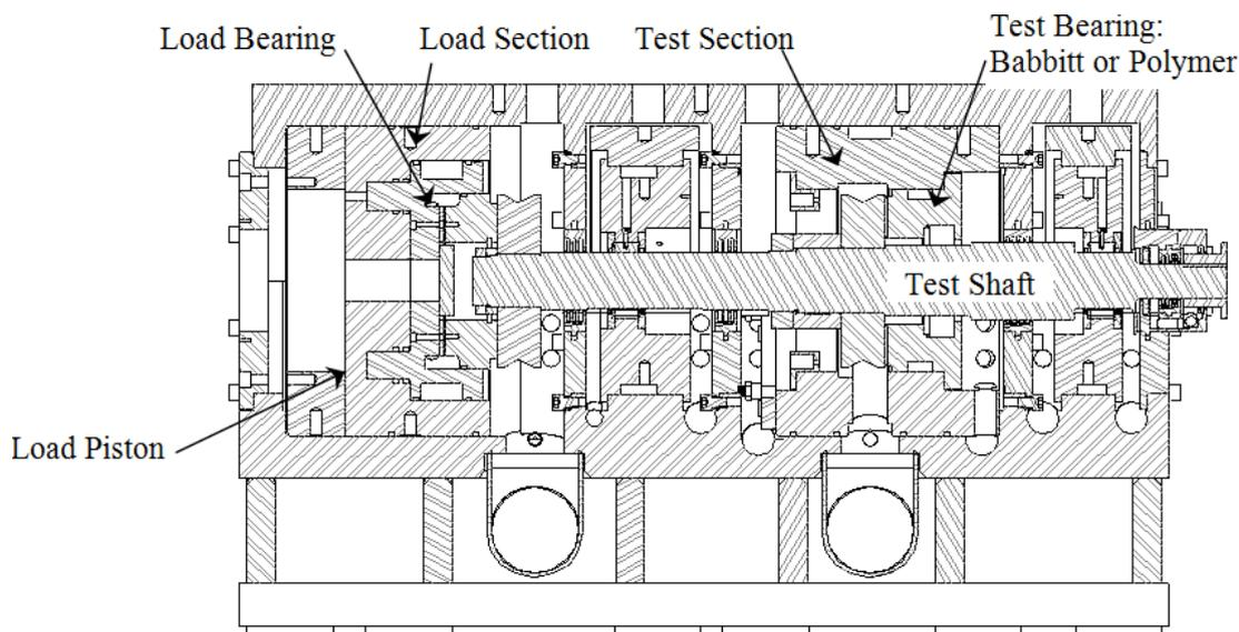
**Figure 1.** Large horizontal thrust rig.
