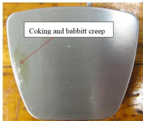
**Figure 6.** Babbitt lined pad after test, 11,000 rpm.
