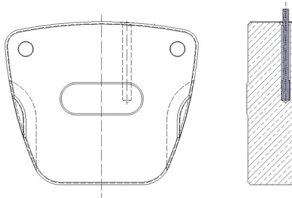
**Figure 3.** Thermocouple configuration.
