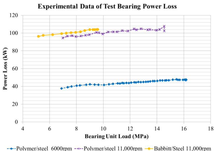
**Figure 8.** Power loss at different speeds.
