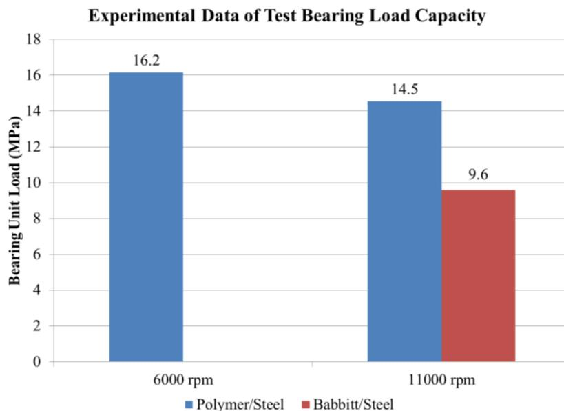
**Figure 4.** Load capacity at different speeds.
