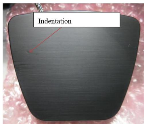
**Figure 7.** PEEK lined pad after test, 6000 rpm.
