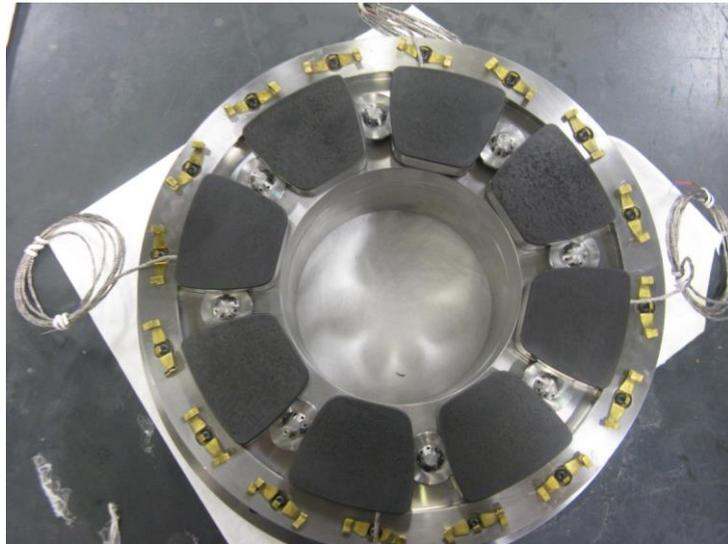
**Figure 2.** Tested tilt thrust bearing with Polyether ether ketone (PEEK) lined pad.
