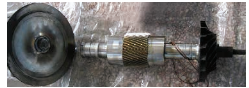
Without ISFD technology: Rotor failure due to increased imbalance from deposits
