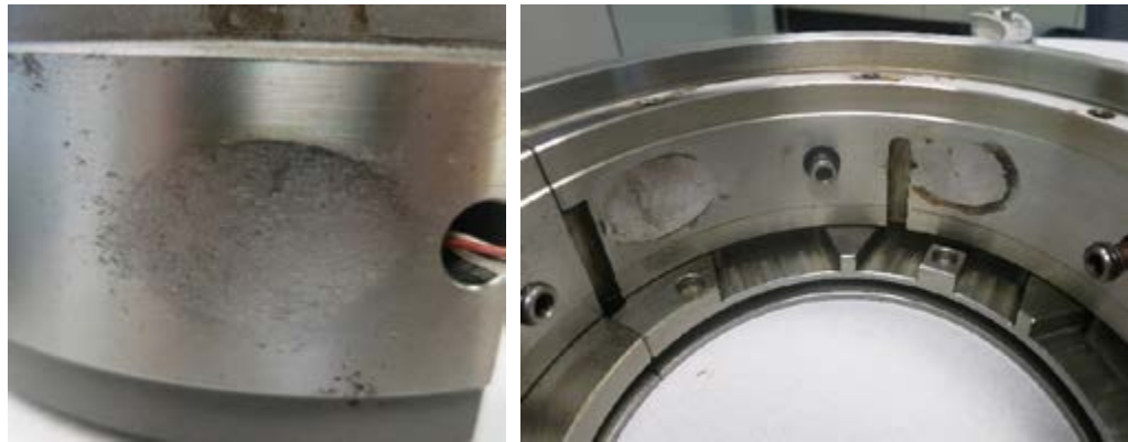
Figure 2: Pivot wear on the point-contact-pivot tilt pad (left) and bearing shell bore (right)
