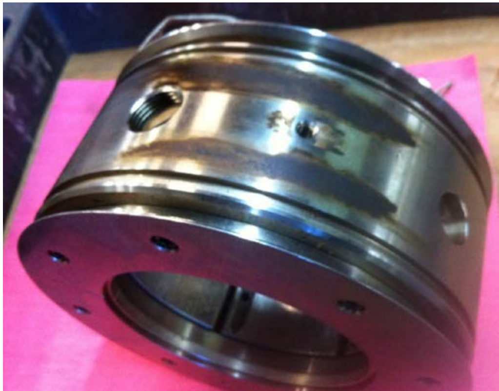
Figure 3: Damage on the OEM bearing outer diameter from bottoming out
