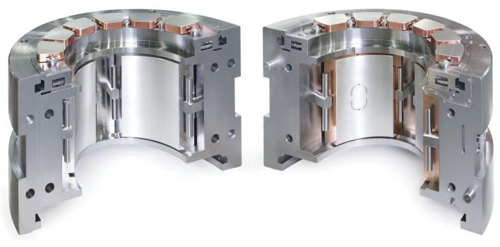
Maxalign bearing using a combination of standard whitemetal lined steel backed pads and whitemetal lined copper chrome backed journal pads with hydrostatic jacking; combined with copper chrome backed thrust pads
