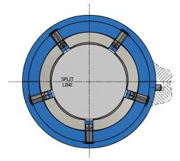
Fig 8 Two-pad orientation – Style BP
