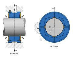
Fig 2 FP series bearing arrangement
