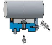
Fig 4(b) Style FL (Minimized leakage at one end)
