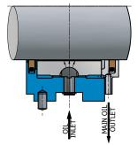
Fig 4(d) Style FL2 (Minimized leakage at both ends)
