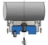
Fig 4(c) Style KN2 (Controlled leakage at both ends)
