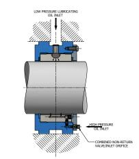
Fig 12 Hydrostatic jacking – Style J
