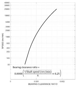
Fig 16 Minimum diametral clearance
