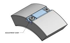
Fig 7 Adjustable pad pivot – Style AP
