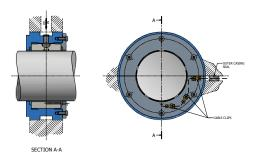
Fig 10 Temperature sensor installation — Style IT2
