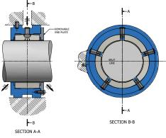
Fig 1(b) TJ series bearing arrangement
