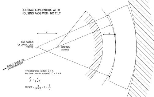
Fig 3 Definition of clearance terms (preset ratio)
