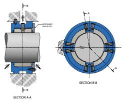
Fig 1(a) TF series bearing arrangement
