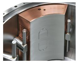
Trailing edge cooling, 'Directed Lubrication' and hydrostatic jacking
