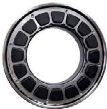
Solid polymer thrust bearings are engineered with temperature capabilities beyond 250 deg C and surface properties allowing for continuous high-load, thin-film operation.
