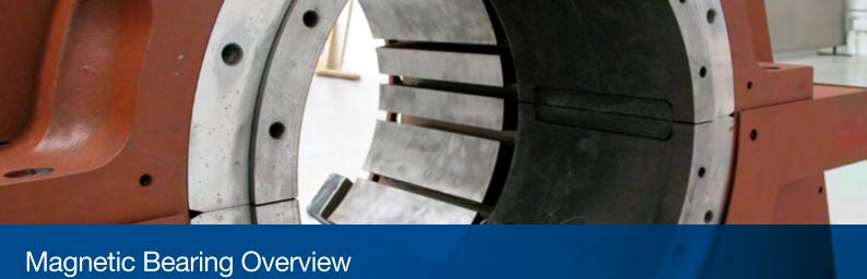
A magnetic bearing is an electromagnetic device used to maintain relative position of a rotating assembly (rotor) to a stationary component (stator). The electromagnetic forces are adjusted in response to forces generated from machine operation using an advanced electronic control system.
